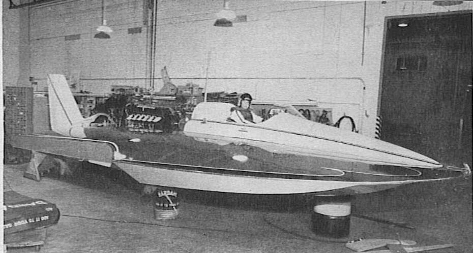
BIG ROLLS engine is swung into place for installation. It'll be covered with a streamlined canopy
